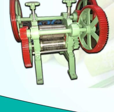
durability. The stainless steel in contact with the sugarcane is food grade steel.
